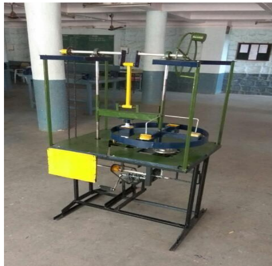
Figure 3: Actual Fabricated Model of special purpose soap stamping machine.
